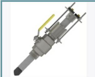
Electromagnetic Insertion Meter for Municipal and Industrial Flow Applications. The SPI Mag Insertion Flow Meter provides a highly cost-effective solution for the accurate measurement of liquid flow in closed conduit, pressurised pipe applications. Unlike conventional magnetic meters, the SPI Mag's cost is independent of pipe size. Velocity and pipe diameter information are utilized by
