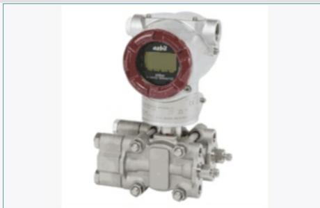
The AT9000 Advanced Transmitters are smart differential pressure and pressure transmitters equipped with microprocessors for high performance and reliability. They can measure flow rate, pressure and liquid levels of gases, liquids and steam, as well as transmitting 4-20mA DC analogue or digital signals in proportion to the measured pressure.
