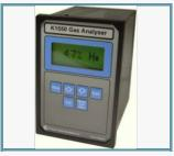
The K1550 accurately measures the changes of one constituent in binary or pseudo-binary gas mixture, i.e. mixtures in which only one constituent changes. Examples include hydrogen, carbon dioxide, argon, helium and various halogenated hydrocarbons such as Freons. Almost any single constituent of a gas mixture can be measured providing its thermal conductivity differs from that of the other components. Ranges from high ppm to 100% are possible depending on the gas being measured.
